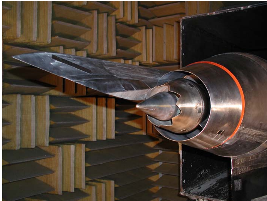
Figure 1. Chevron nozzle with pylon, installed in the NASA Langley Low Speed Aeroacoustic Wind Tunnel (from Thomas and Kinzie [53])
