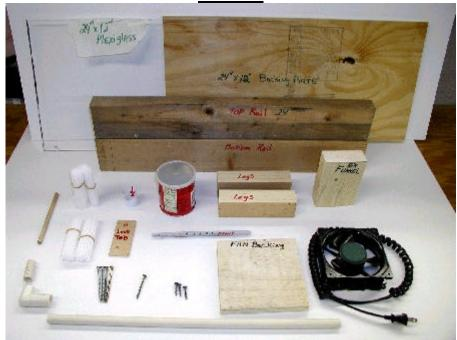
NOTE: You will purchase your plastic pipes based on the Inside Diameter (ID) (Ex.  $\frac{1}{2}$ " ID plastic pipe), but you will be drilling based on the Outside Diameter (OD) (Ex.  $\frac{5}{8}$ " OD, which may vary). So if there is any uncertainty, MEASURE before drilling a hole.
