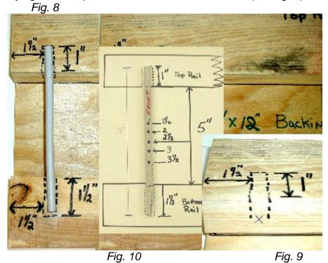
**Step 15a:** Trace the outline on the wood as shown in Fig. 8. Mark the inner edges of the tunnel on the tube (this will help during construction).
