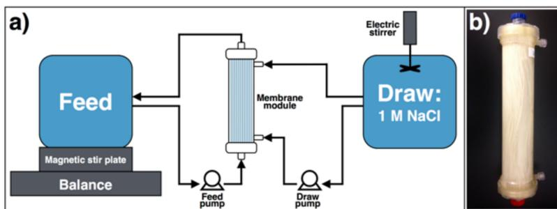
▲ (a) Schematic overview of the FO setup and (b) an image of the membrane module used in this study
