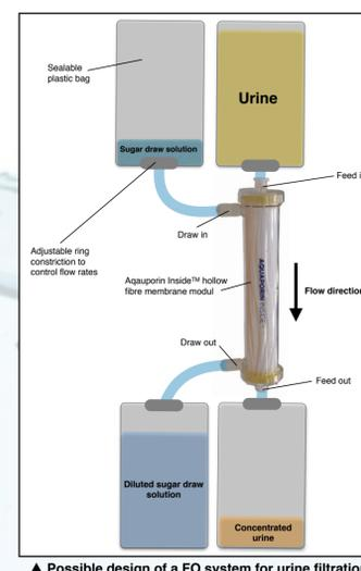
▲ Possible design of a FO system for urine filtration
