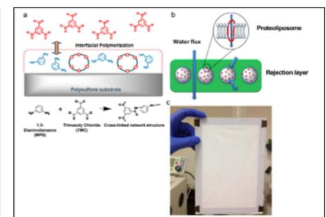
▲ The manufacturing process of an aquaporin-based membrane [17]
