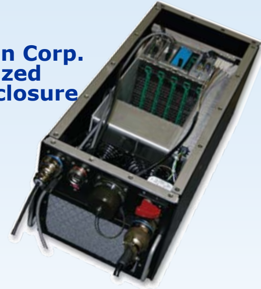
microTCA conduction cooling concept development
